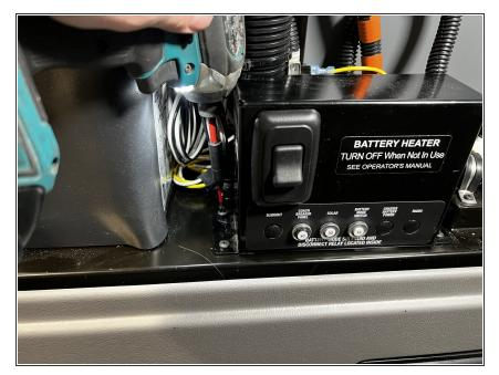
Place the breaker panel back into the battery compartment, and reinstall using the screws removed previously to secure it to the compartment.
