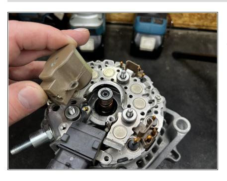
With the 4 screws removed securing the internal regulator and the brush cap, lift the brush cap off and set aside.
