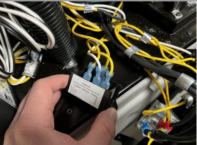
Located the combiner behind the breaker box. Using a #2 Phillips bit, remove the screws securing the combiner.
