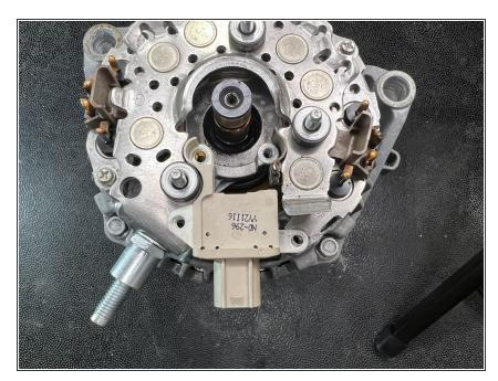
Take the new terminal block provided in the kit and place onto the alternator as shown.
