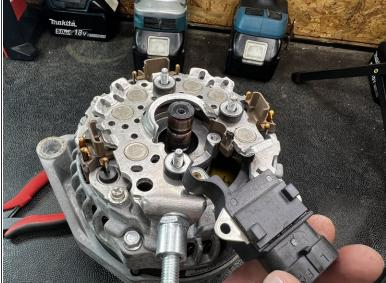
With the solder joint cut free, lift up on the internal regulator and remove from the alternator. This
