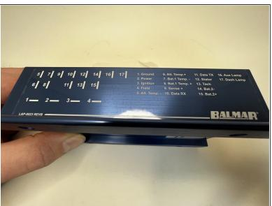
This is the pin out diagram for the Balmar regulator. This will be needed in the coming steps.
