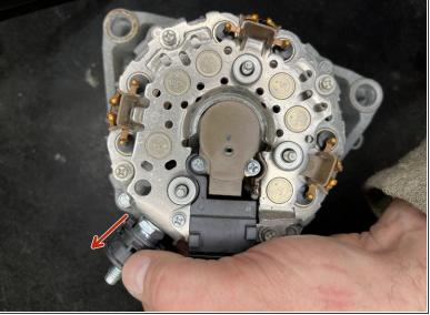
Slide the plastic sleeve off the positive stud, and set aside.
