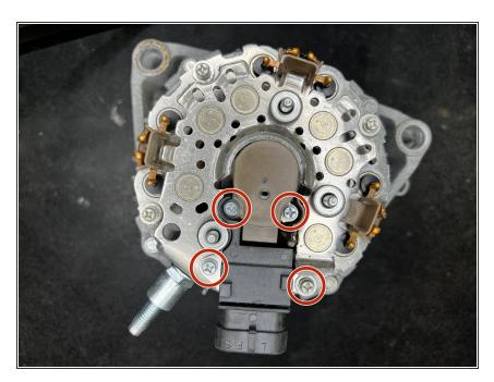
Locate the 4 Phillips head screws that secure the brush cap and regulator onto the alternator.
