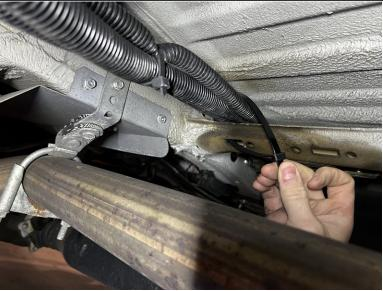
Since we removed rear-most clamp, secure the wire bundle the rear crossmember support using a provided zip tie.
