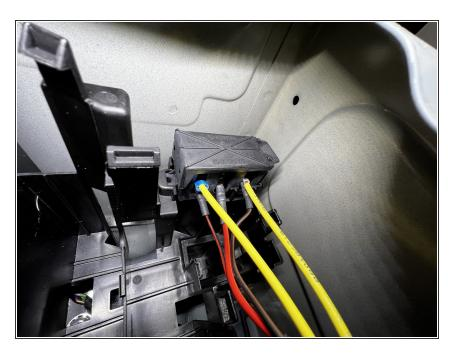
Remove the EK1 module by pushing the locking tab (near the rear of the seat base) to the rear of the van, and lifting the right side of the EK1 up to slide it out of the mount.
