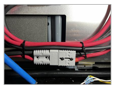
With the insulated clamps installed, used the provided zip ties to secure the other battery cables for the 2 upper batteries as shown.
