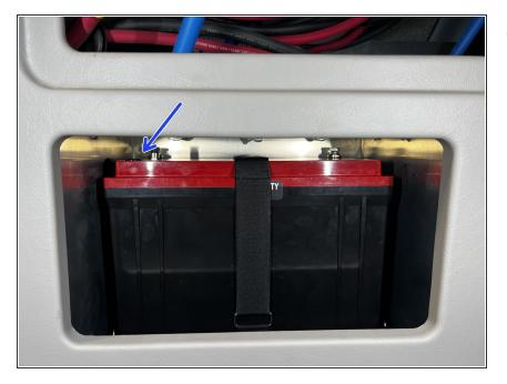
If equipped with a 3rd battery, the ON/OFF switch will be located on the front left corner of the battery. Depress for 5 seconds to turn the battery off.
