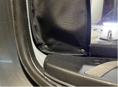
Reinstall the screen into place, an secure using the screws removed previously.
