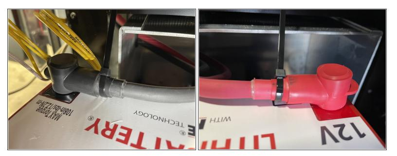
With the cables secured to the battery terminals and the protective boots installed, install one of the provided zip ties on each protective boot. This will prevent the boot from sliding off, and exposing the battery terminal. Cut the tails off the zip ties once secured.
