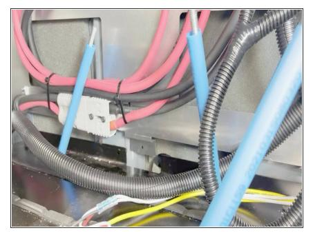
In most cases the screws securing the shelf are stripped. Mark new screw positions next to the holes already in the shelf. Do this for all the mounting points on the shelf.
