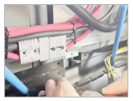
Install the provided self drilling screws to secure the battery shelf to the van.
