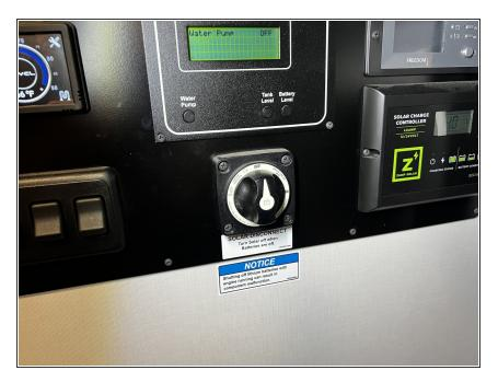
Turn the solar disconnect knob located on the control panel to the "OFF" position.
