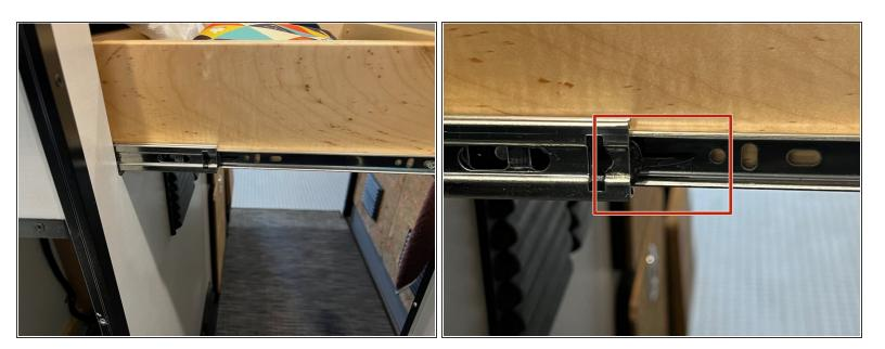
Remove the top drawer from the galley by sliding the drawer all the way out, and depressing the black release tabs on both drawer slides and pulling the drawer out. Set the drawer aside.
