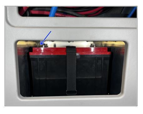
If equipped with a 3rd battery, the ON/OFF switch will be located on the front left corner of the battery.
