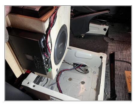
With all the wiring connections disconnected, the sub box may now be lifted and removed from the seat base and set on a bench to finish the update.
