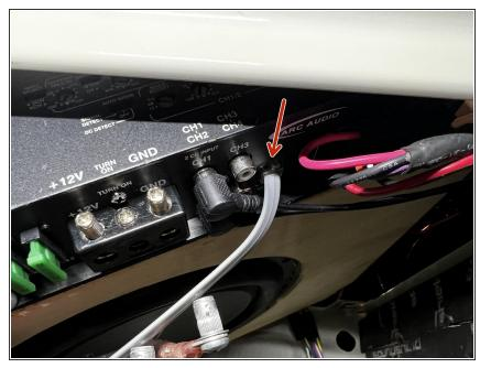
Unplug the RJ12 cable for the bass control knob from the amplifier.
