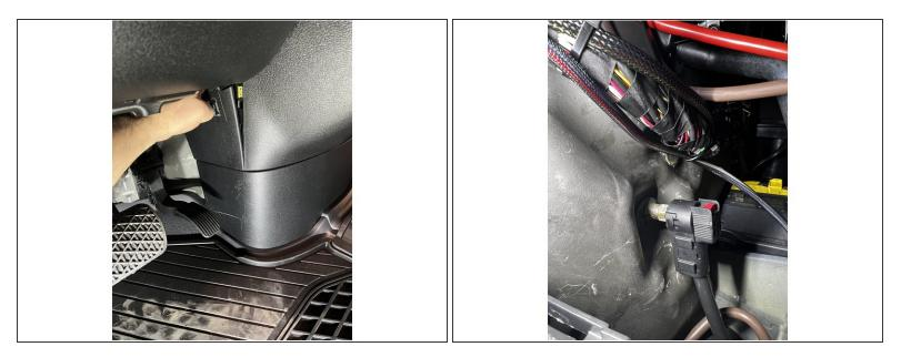
• Remove battery ground disconnect access cover to expose battery ground disconnect
