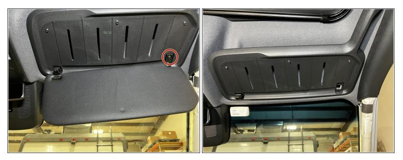
Unclip the visor from the visor shelf. Using a T30 Torx bit to remove the screw securing the visor to the visor shelf.
