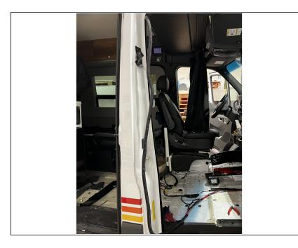
• Pull the fuse panel wire harness out from behind the B pillar trim as shown. There may be some zip ties securing the harness inside the B pillar. You will need to cut those zip ties if that is the case.
