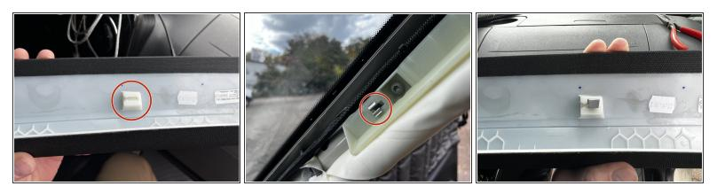
• In some cases this metal tab will be left on the vehicle side. Remove it using a pair of pliers and reinstall it onto the A pillar trim.
