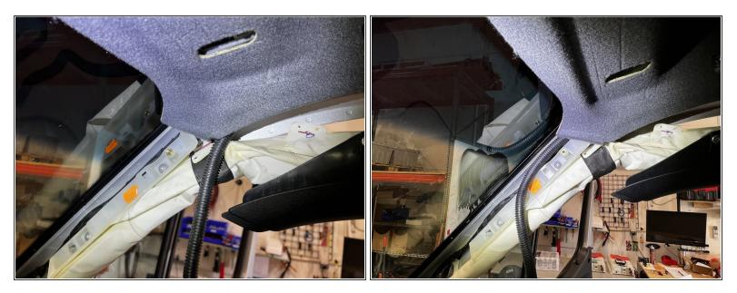
• With the harness routed forward, bring it to the A pillar. Route the harness above the airbag, and in between the headliner and the plastic airbag mounting bracket.
