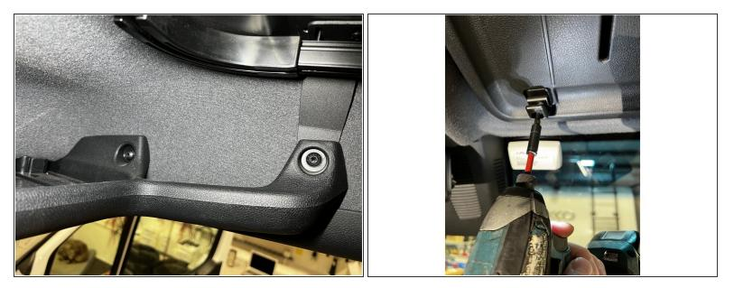
• Reinstall the visor shelf back into place using the T30 Torx screws previously removed.
