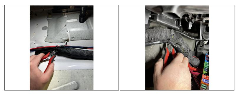
• Cut any zip ties securing the fuse panel wiring bundle to the OEM Mercedes wiring loom. The fuse panel wiring bundle runs up to the fuse panel under the passenger side of the dash.
