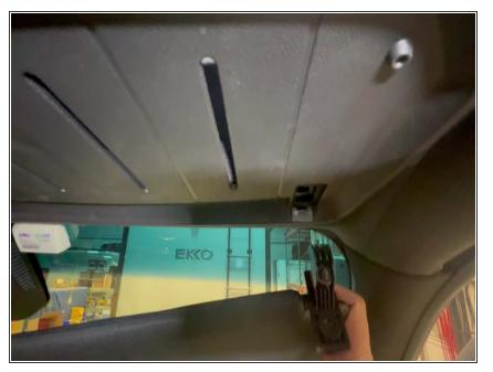
Hook the visor into the slot, then roll the visor into position. Then push it forward to get it to seat properly into the visor shelf. Once it is hooked in seated, the screw can be installed.
